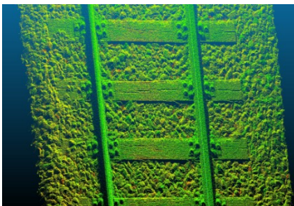
3D image taken by the Rail Track Scanner RTS developed by Fraunhofer IPM. Picture courtesy of: iNovitas AG, www.inovitas.ch
