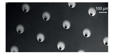
Vias in printed circuit boards have to be drilled with micrometer precision. A new measuring method is set to make it possible to control the microvias laser drilling process. (Image: 3D-Micromac AG)
