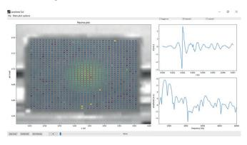
Test measurement on a concrete cube measuring 50 cm × 50 cm: AI-based software developed by Fraunhofer IGP identifies conspicuous measuring points, localizes areas of damage and immediately visualizes the results. Individual measuring points are visible; their color provides information about the intensity of the vibration. Bright areas indicate delamination in the center of the specimen. Each measurement signal can also be displayed in detail as a graph. © Fraunhofer IGP
