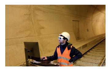
Damage to concrete structures is often hidden underneath the surface. With laser-induced vibrations, these subsurface defects can be efficiently detected and automatically evaluated – more accurately than the common impact hammer test can. Measurements have shown that this also works under real conditions inside a tunnel (here, underground research facility ZaB, Austria). © Jannis Gangelhoff / Fraunhofer IPM
