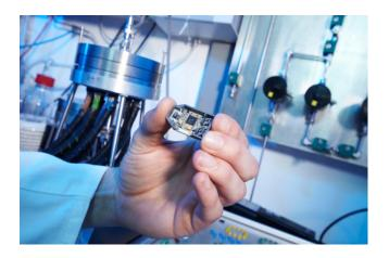
In Fraunhofer IPM's sensor, dyes react to gases – and trigger an alarm, even in the case of smoldering fires. (© K.-U. Wudtke/Fraunhofer IPM) | Picture in color and printing quality: www.fraunhofer.de/press
