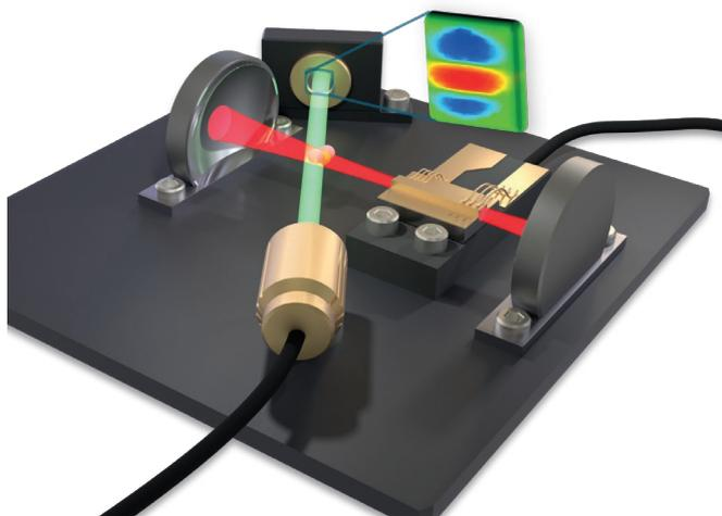
**Measuring principle of photothermal spectroscopy:** A laser beam (red) is directed at the target substance and is absorbed by its molecules as heat is released. Local heating produces a characteristic pattern in a second probe laser beam (green), which looks similar to a heat flicker (magnified). This pattern can be detected with high sensitivity.
