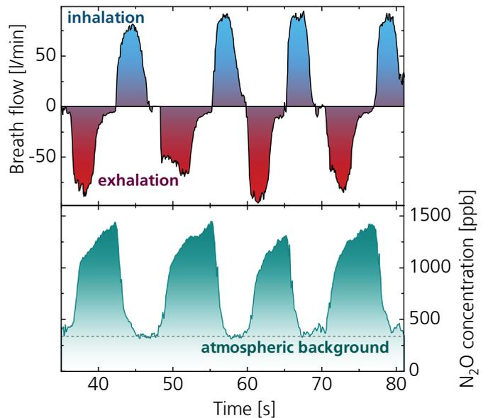
*Example measurement: Nitrous oxide (N<sub>2</sub>O) as a metabolic product in the respiratory air. The MVP gas analyzer simultaneously measures the respiratory flow and the concentration of trace elements.*
