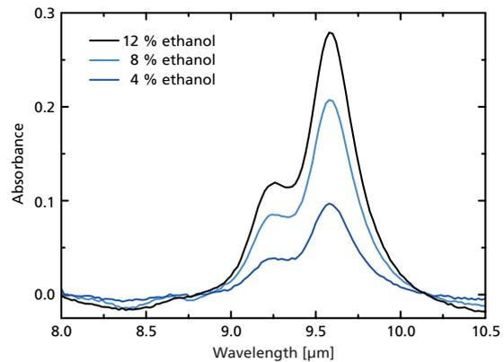
**Measured spectra of different ethanol concentrations with spectrally tunable pyroelectric detector.**
