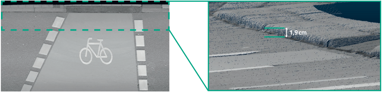
Left: The dense point cloud acquired by the PPS provides a photorealistic image of the road surface (grayscale value = backscattered intensity). Right: The 3D data allows precise measurement of the road surface.
