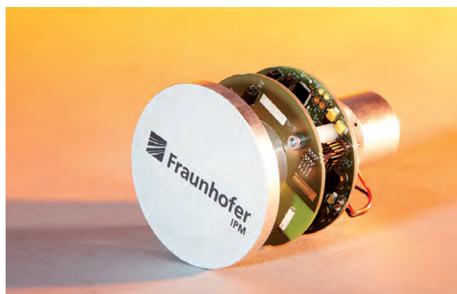
An energy-autarkic sensor supplies enough energy to measure the temperature and quantity of coffee and to transmit the data by radio signal to a PC.
