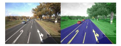
The deep learning framework by Fraunhofer IPM can automatically detect trained objects in real time and displays them with a color mask (right). © Fraunhofer IPM
