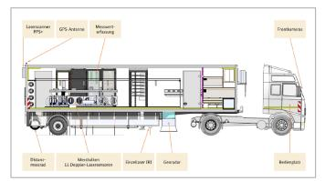
MESAS features various mainly laser-based measuring systems which record the road surface without contact. The measurement data are synchronized and georeferenced with the help of a GNSS system. Software tailored to the applicatoin manages the data and supports route planning and quality assurance during operation.
