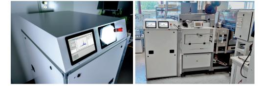
Fraunhofer IPM and Fraunhofer ISIT have developed an inline measurement system based on LIBS technology that quantitatively measures the chemical composition of coated electrode foils on a point-by-point basis using a form of 3D mapping (I.). The measurement system was recently integrated into the laboratory plant of an electrode manufacturing facility at Fraunhofer ISIT and tested (r.). © Fraunhofer IPM
