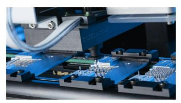
The semi-automatic pilot production facility for thermoelectric high-temperature modules, developed by Fraunhofer IPM, allows far larger quantities than before – and with the same high quality. © Fraunhofer IPM, Germany.
