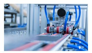
The fuel cell stacking process is very complex: The image shows a membrane electrode assembly (MEA) with gas diffusion layer (GDL) being transported. Image: © thyssenkrupp
