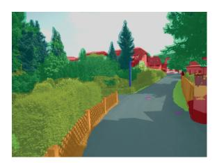
Textured point cloud generated from camera images and laser scanner data. An Al-based algorithm recognizes, classifies and codes individual object classes in color. Object information automatically feeds in to smart planning maps which then form a basis for infrastructure planning. (© Fraunhofer IPM
