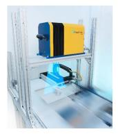
The fluorescence scanner – an imaging, inline measuring system – inspects components for impurities during the manufacturing process and identifies the exact point of contamination. Photo © Fraunhofer IPM <u>www.ipm.fraunhofer.de</u>.
