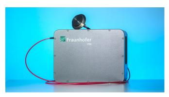
F-Fiber: The fiber-based fluorescence sensor allows for insights into closed vessels. The millimeter-fine fiber probe is integrated into the container wall via a flange and measures the degree of fouling. This way, cleaning routines can be dynamically adjusted according to the actual amount of deposit present.
