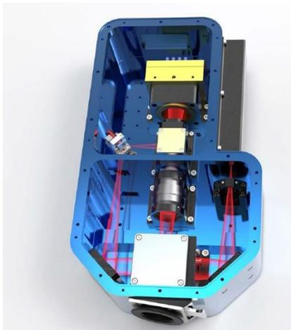
The system can measure centimeter-sized rough objects in fractions of a second with micrometer accuracy – even under disturbances, such as vibrations. © Fraunhofer IPM |
