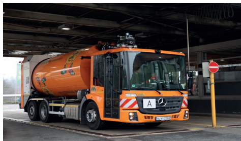
Garbage collection and measurement vehicle in one: with the compact and robust sensor box on the roof, every vehicle becomes a measurement vehicle.© AWG Wuppertal
