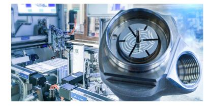
Identifying a single component out of thousands: Using the Track & Trace fingerprint technology, mass-produced components such as this component of a highperformance injector can be reliably identified in the production process without having to be marked. In this way, production data can be assigned to individual components for optimized production. (*Picture: Bosch / montage Fraunhofer IPM*)
