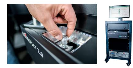
The Ratiospect 2.0 measuring system allows for a much quicker, more accurate and more sensitive measurement of lightsensitive plant protein concentrations. © Fraunhofer IPM
