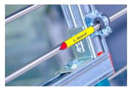
Continuous, comprehensive detection of even minor leaks is a prerequisite for safe hydrogen infrastructure. Sensor technology is destined to occupy a key role here – for example when it comes to upgrading the existing natural gas grid to allow the transportation of H<sub>2</sub>. (© Fraunhofer IPM) **PRESS RELEASE** June 9, 2022 || page 2 | 3
