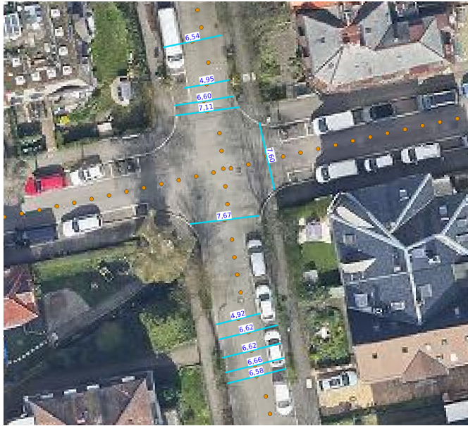
Fig. 2 Automatically collected street width data displayed as an overlay in a geographical information system
