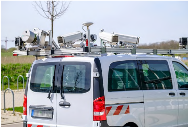
Fig. 4 Survey vehicle equipped with cameras and sensors from Fraunhofer IPM
