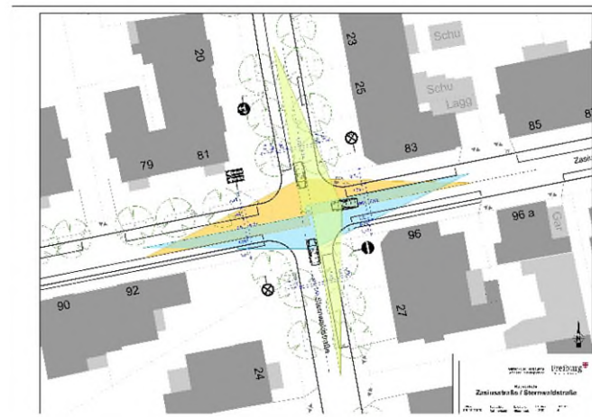
Fig. 3 Complex intersection with different street widths. The data was collected manually, added to a plan and served as a reference for development
