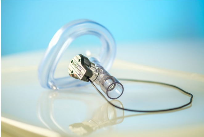
Fig. 1 The noninvasive miniature sensor can be incorporated into existing ventilation equipment via a T-connector.
