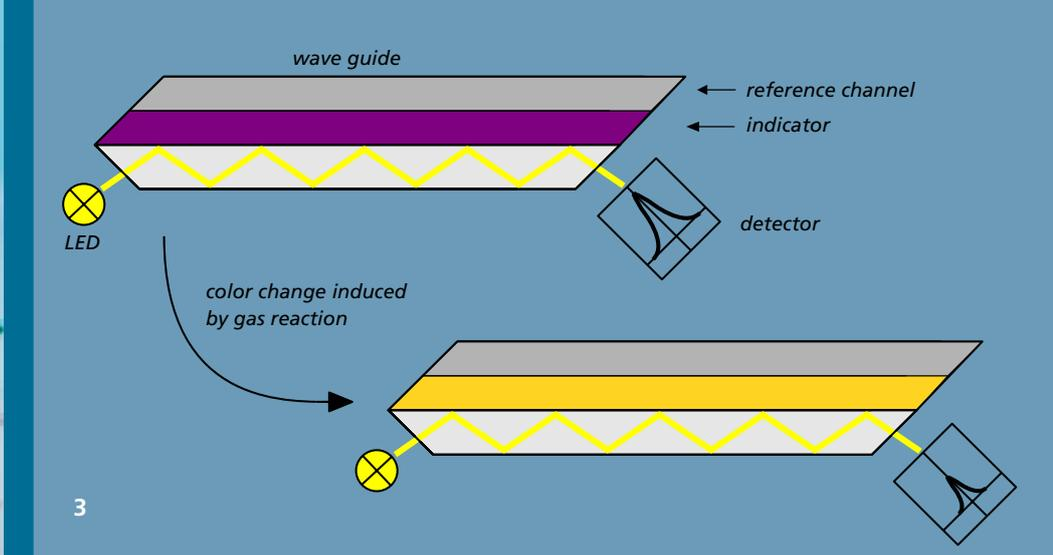
signal is generated from the change in voltage in the photodiode. For the purposes of stabilization, the sensitive material is embedded in a polymer. This polymer dye matrix is applied to the waveguide using microsystem technology methods – e.g. spin coating, screen printing or inkjet printing. The research focus at Fraunhofer IPM is on the development of colorimetric sensors with reversible color reaction.
