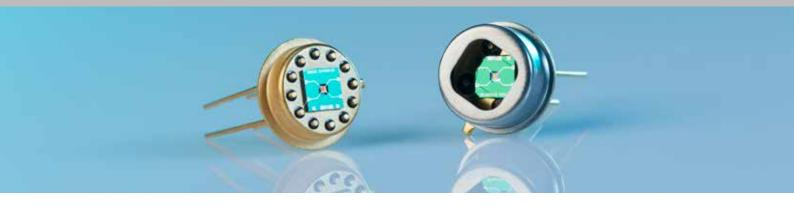
∧ Micro-structured, modulated IR emitter: The emitting surface is freely suspended in the chip.
