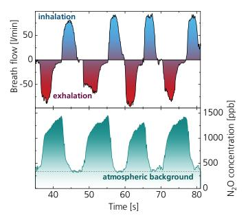
**Example measurement:** Nitrous oxide ( $N_2O$ ) as a metabolic product in the respiratory air. The MVP gas analyzer simultaneously measures the respiratory flow and the concentration of trace elements.
