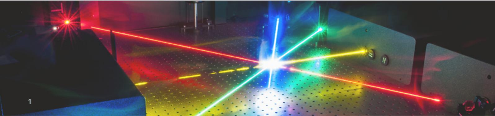
1 *Nonlinear optics for tailor-made light output, developed and built at Fraunhofer IPM: crossed beams of four continuous-wave optical parametric oscillators tuned to different wavelengths in the visible range.*
