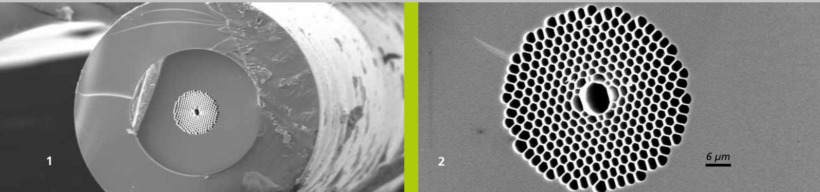
1 *Hollow-core photonic crystal fiber: The sample gas and the Raman excitation laser are coupled into the inner core of the fiber.*
