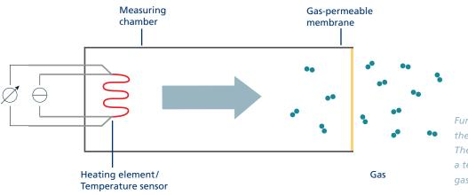
Functional principle of a thermal conductivity detector: The heating element serves as a temperature sensor of the gas matrix.
