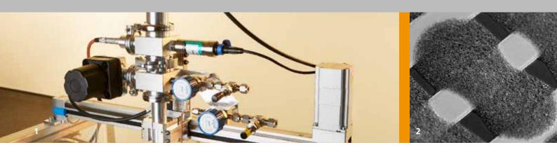
1 Measurement setup to characterize and optimize the semiconductor material at temperatures of 20 to 800°C.
