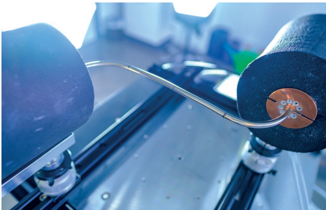
The heat pipe measuring station is specially designed to characterize tubular heat pipes. We examine heat pipes with different diameters, lengths, and bends, as well as adjustable tilt angles and spatial orientations.
