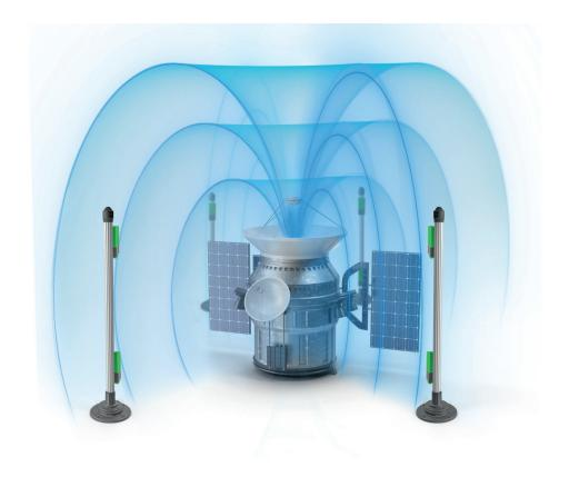
Estimating residual magnetization from stray-field measurements: sensitive magnetometers sample the satellite's magnetic field at multiple locations. These data are used to solve an inverse problem (e.g. regularized dipole/ multipole fitting) in order to reconstruct the spacecraft's equivalent magnetic sources. The solution yields the magnitude and direction (with uncertainty) of the magnetic moment that best explains the measured field.
