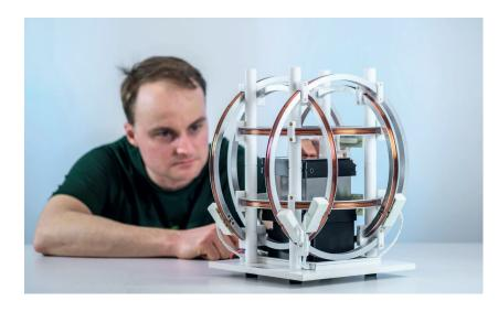
The performance of new shielding materials is tested in an experimental setup. Here, a cube made of mu-metal plates is placed at the center of a 3-axis Helmholtz coil system.
