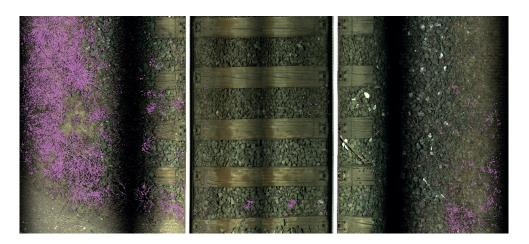
Vegetation detection on a track bed: Measurements can be taken at travelling speeds of up to 100 up km/h. The vegetation (depicted in purple) is visible in detail. The command to apply the herbicide is executed specifically on the basis of threshold values.
