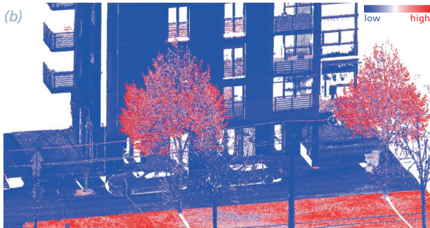
Above: The CPS' scanning data provides information on objects interfering with the clearance profile (marked red).
