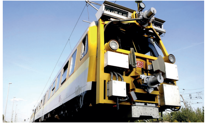
Right: HSP system with two sensor heads mounted on the Deutsche Bahn inspection train LIMEZ III
