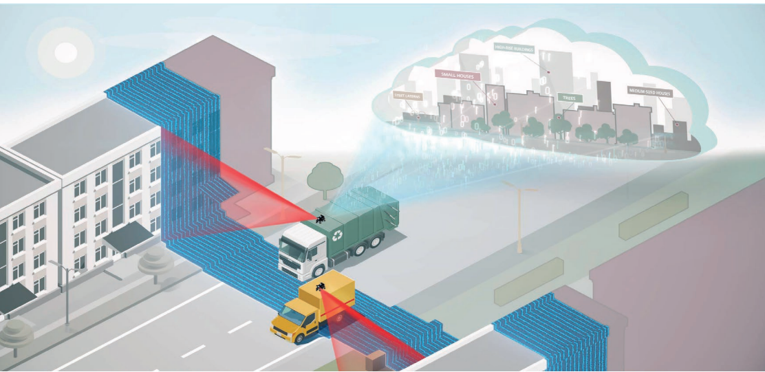
MUM mini turns conventional vehicles into measurement vehicles: These vehicles map the environment and provide evaluated, classified measurement data in real time.
