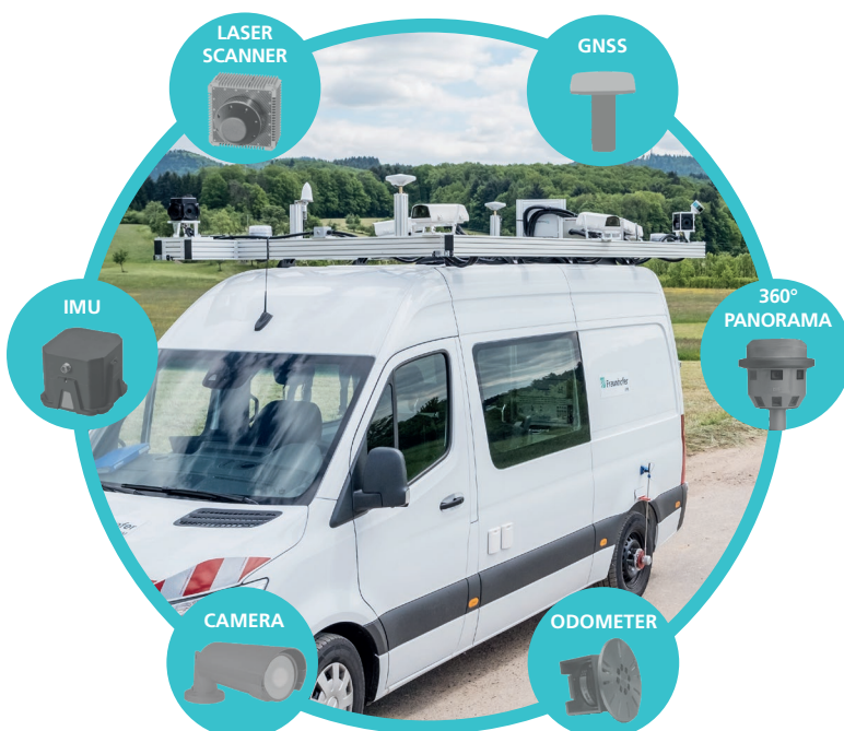
Typical sensor stack for a MUM system.
