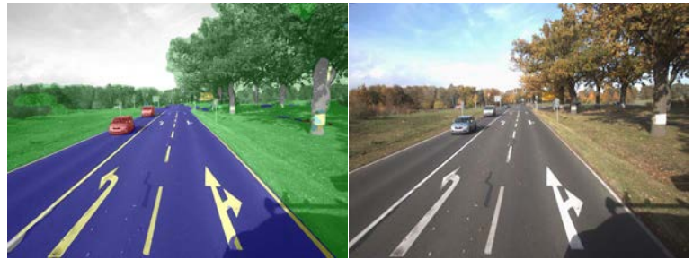
Camera image and evaluated measurement image: Colored segmentation masks mark the forms of the identified objects.
