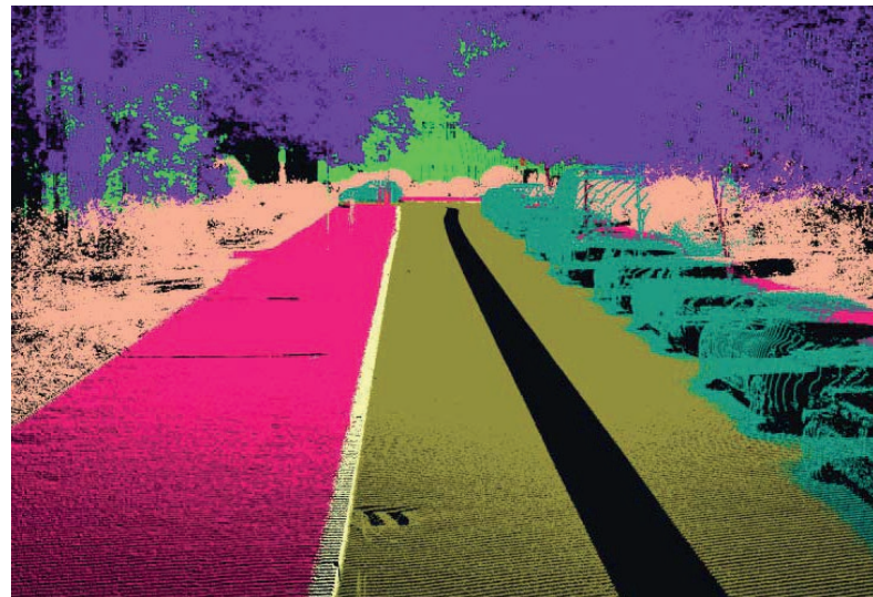
Left: Textured point cloud, reconstructed from data taken at 50 km/h with a CPS laser scanner and four cameras.
