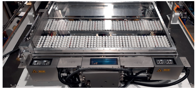
The CIS with open lid showing the individual sensors: The CRS (middle bottom), two LPS (left and right bottom), and LED panels for illumination. The cameras for wire wear measurement are located between the LED panels (not visible). The metal rails are used for the semi-automatic cleaning system.
