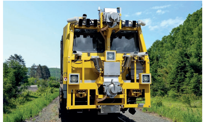
Right: The two sensor heads of the HSP mounted on the Deutsche Bahn GMTZ inspection train.
