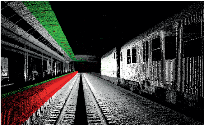
Left: Image based on profiles taken with the HSP to analyze clearance.
