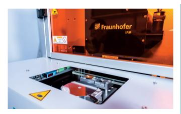
HoloAMS is set up with application-specific sensors and actuators to solve the measurement task reliably and economically. Components can be fed into the system manually or automatically by a robot.
