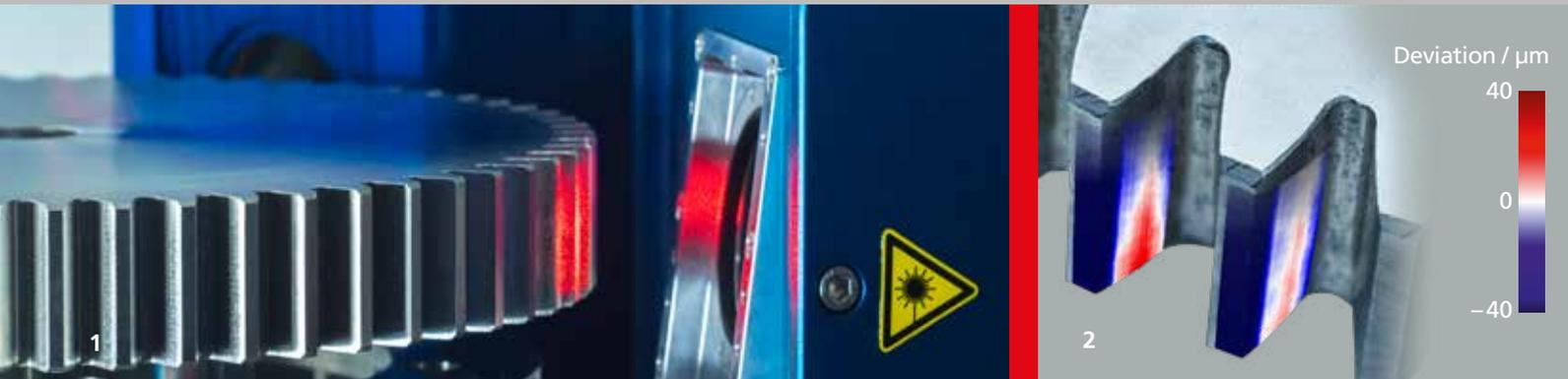
**1** The digital holographic measurement system HoloGear captures the entire surface of gear geometries – faster and with greater precision than any other measurement system in the world.
