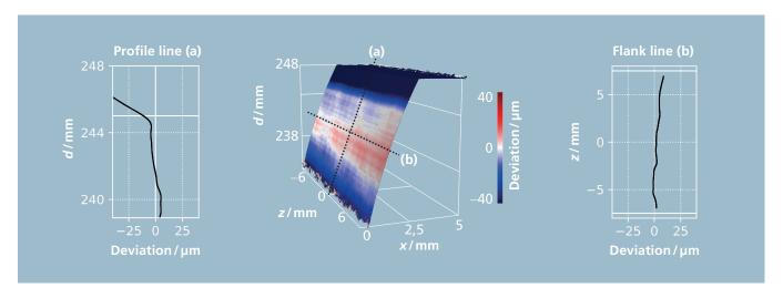
HoloGear captures the entire tooth flank of an involute gear (incl. the addendum circle) in a single shot in less than 200 ms. The picture shows an example gear with 248 mm outer diameter, module 4 and a tooth width of 15 mm. 3.6 million 3D points are captured on one flank.
