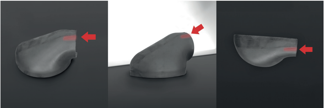
As with visual inspection, components – here a formed sheet metal component – are inspected from several perspectives. The automated image evaluation shows typical defects such as cracks, scratches or dents.
