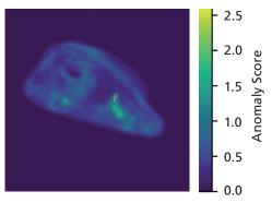
Inspect-360° MP detects defects in places that were previously difficult to inspect automatically – regardless of the orientation and position of the component. The scratch above the hole is reliably detected. The color indicates the deviation from the nominal value.
