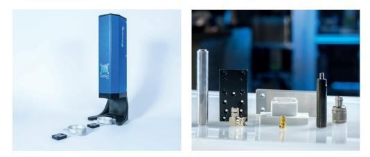
The portable Track & Trace Fingerprint Flex system measures 30 cm in height and 10 cm in width. It is suitable for sample component authentication at varying locations.
