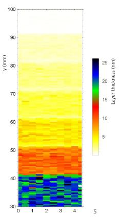
5 Aluminium sheet with locally different coating thickness bet-ween 1 and 20 nm.
