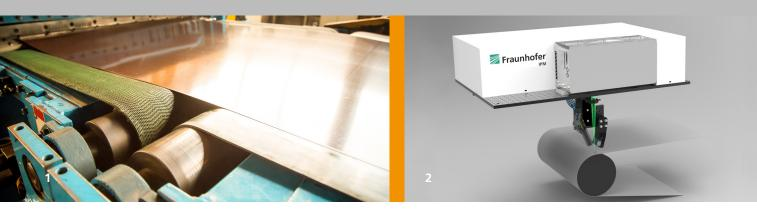
Corrosion protection coatings on metal strips should be homogeneous and coat the metal completely. The ANALIZEsingle measurement system measures nanometer-thick layers during the coating process.
