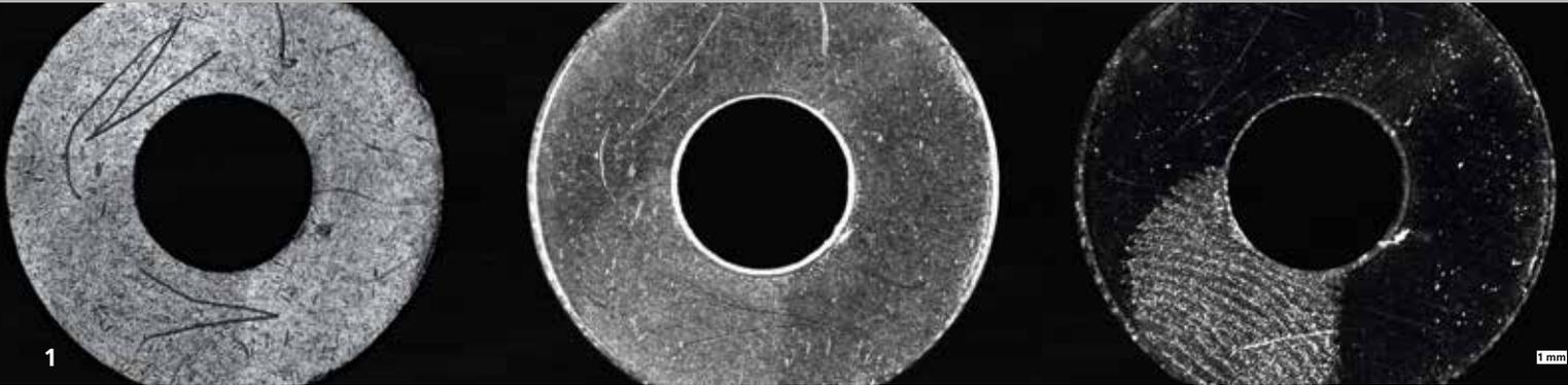
1 Three imaging methods for inspecting for defects and contamination: bright field (left) and dark field (mid) reveal shape defects, particles and scratches. Fluorescence reveals organic contamination (right).
